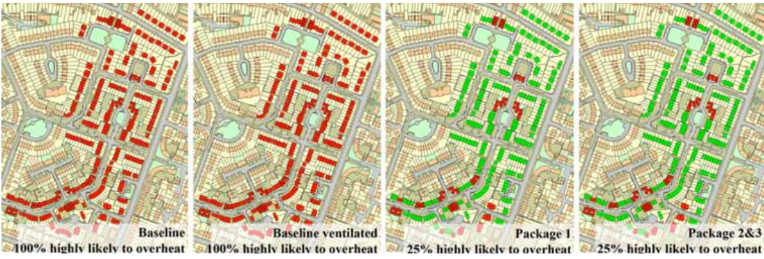
Figure 7.6 Adaptation package results for 2050s, high emissions, 90% probability in Upper Horfield. Note: packages 2 and 3 do not differ in overheating reduction as package 3 is defined by the inclusion of solar energy systems alone (source: Digimap, 2012; The DECoRuM-Adapt model, 2012). Models reproduced under the terms of the Contractor's Licence for the Use of Ordnance Survey Data between UWE, Bristol and Bristol City Council. Map© Crown Copyright/database right 2012. An Ordnance Survey/EDINA supplied service.
